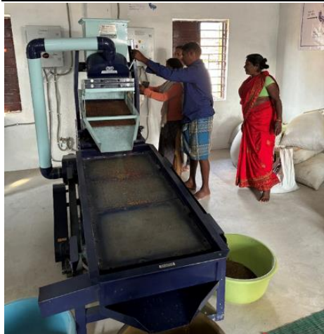
Solar run grain filtering machine, Navatoli
